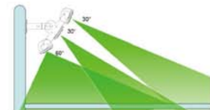
With rotatable LED module for 11 different angle settings to fulfill all spot lighting needs
